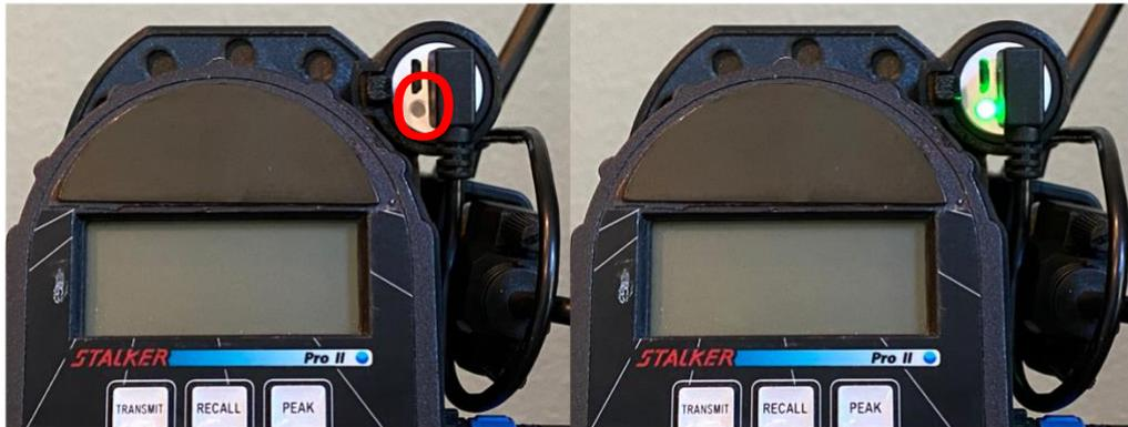
3. A Red and Blue light will come on indicating that the Adapter is powered on. The Red light will be solid the Blue light will blink on and off.
