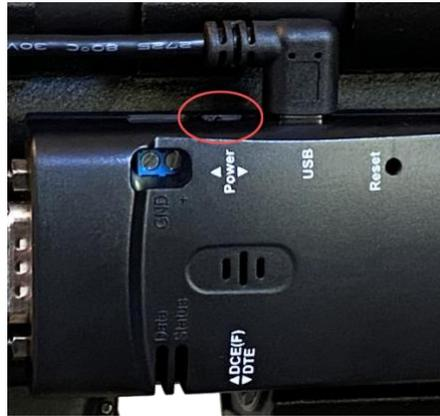
2. Power on the Anker battery. **Push this button.** A green light will appear if the battery is fully charged. If the light is amber in color the battery needs to be charged. Your YJC Wi-Fi Adapter will run for 14 hours off a fully charged battery.
